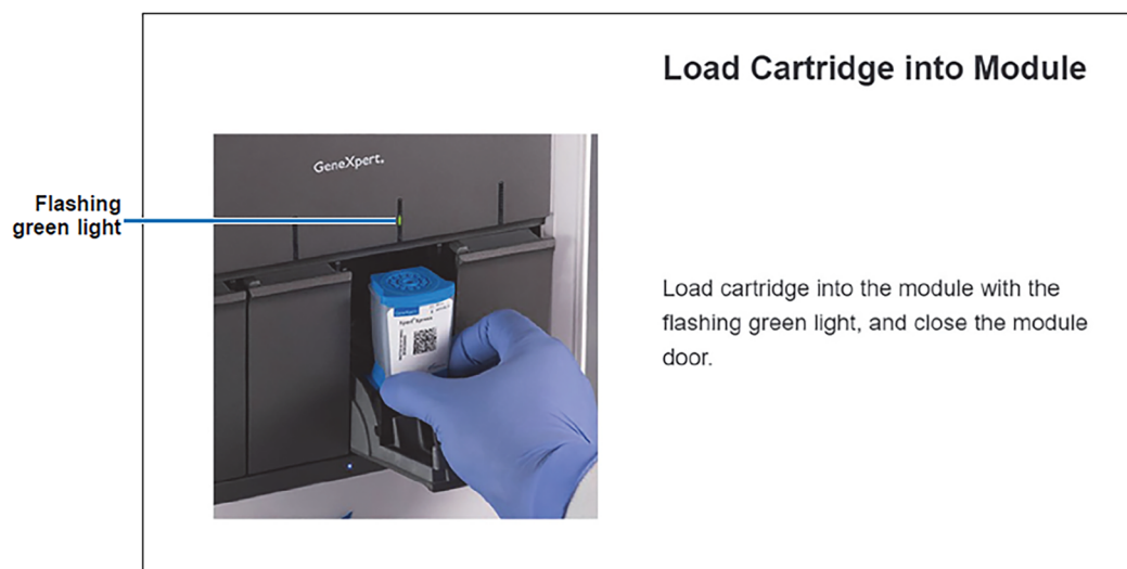
Figure 12. Load Cartridge into Module Screen
